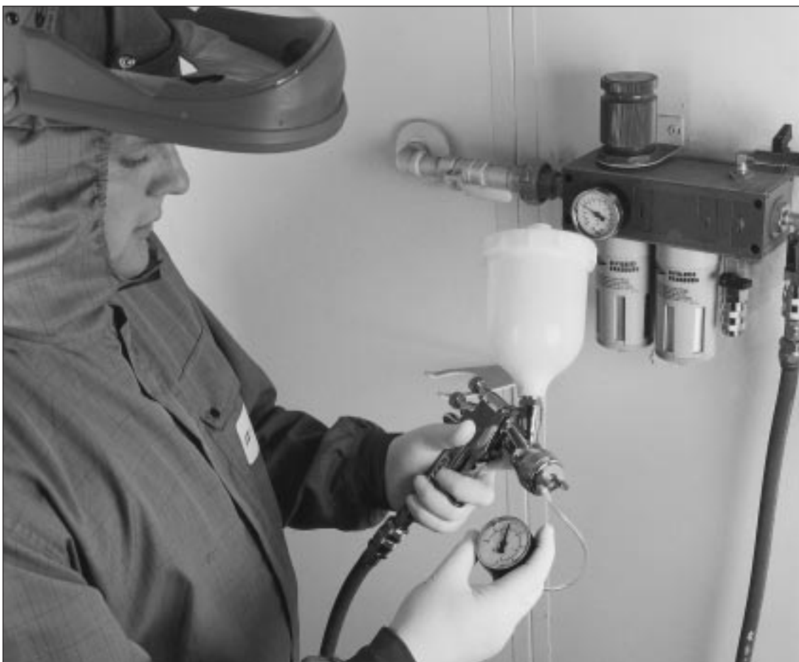
Checking air pressure on an HVLP gun
