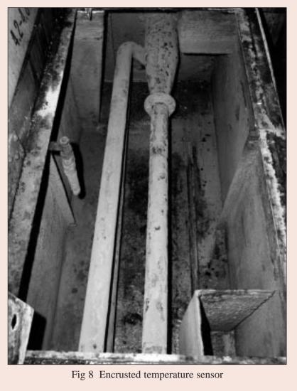
An additional 1°C rise in solution temperature uses about 5% extra heat energy.
