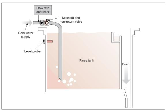
Fig 7 Typical flow controller arrangement
