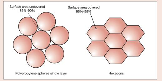
Fig 6 Comparison between single layers of polypropylene spheres and hexagons
