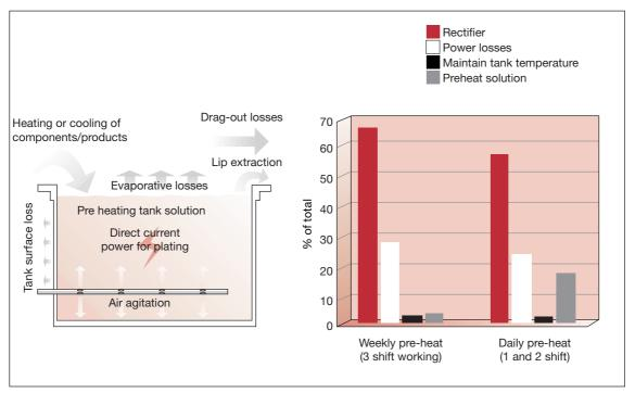
In a typical plating/anodising tank energy is used (or lost) in the ways illustrated in Fig 4.
