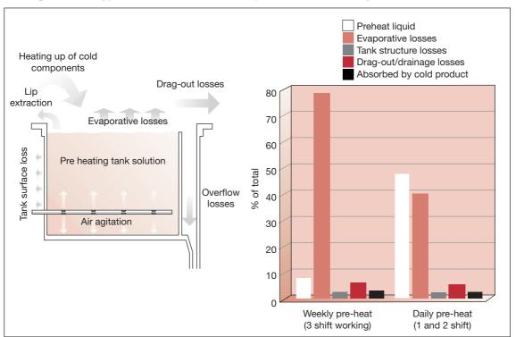
Fig 2 Typical breakdown of heat energy use for a dip tank
