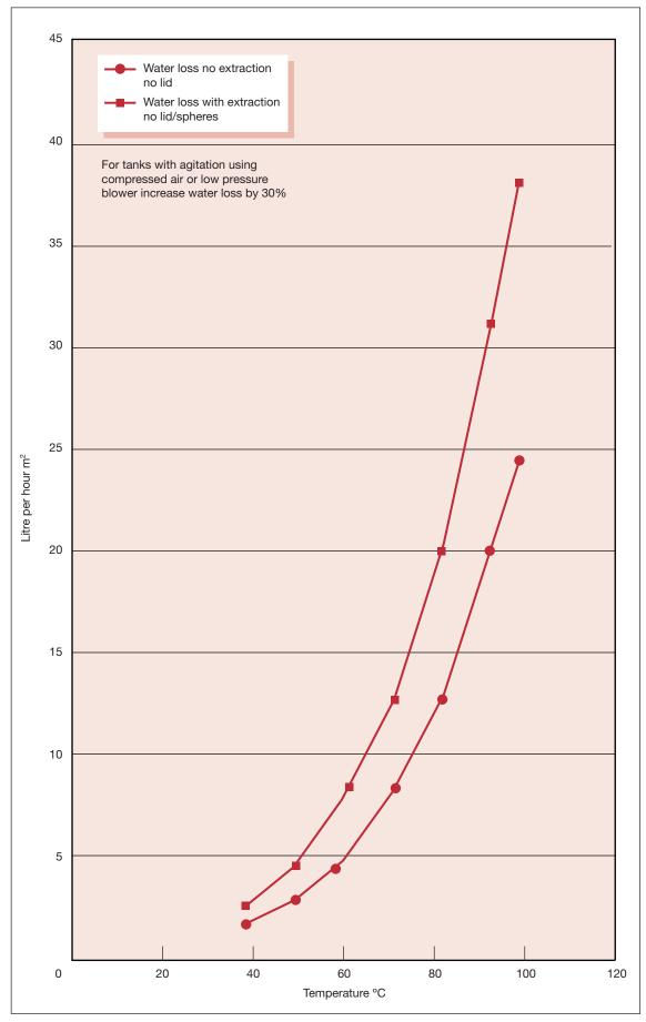
Fig 5b Evaporative water loss from tanks
