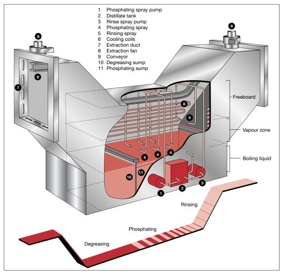
Fig 1 Diagram of typical spray rinsing tank
