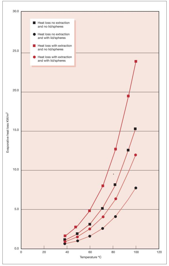
Fig 5a Evaporative heat loss from tanks with extraction and lids/spheres
