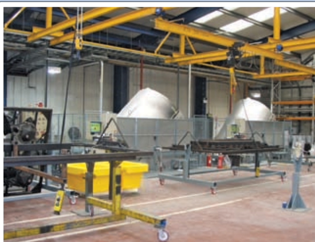
Two-axis rocking rotational moulding machines at XJF Plastics that benefit from excellent Lanemark burner control built into the Sorcerer Machinery design.
