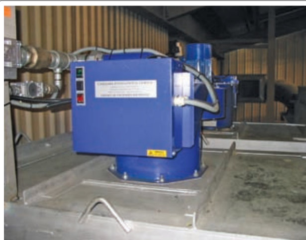
A Lanemark burner used by RotoMech which fires vertically down into the moulding oven.
