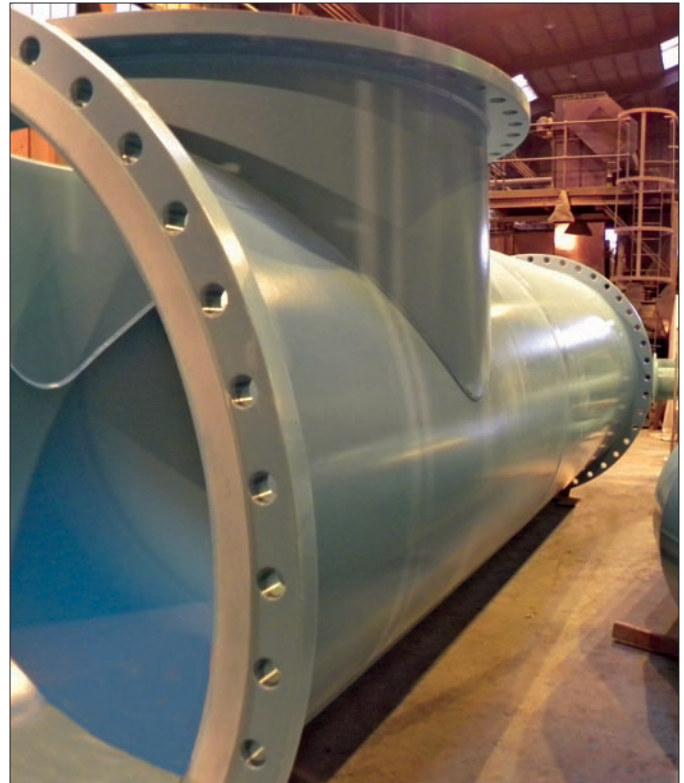
The powder coating of water processing pipes is a key part of Northpoint’s work – and now benefits from Lanemark’s gas and air burners (as shown on reverse).
