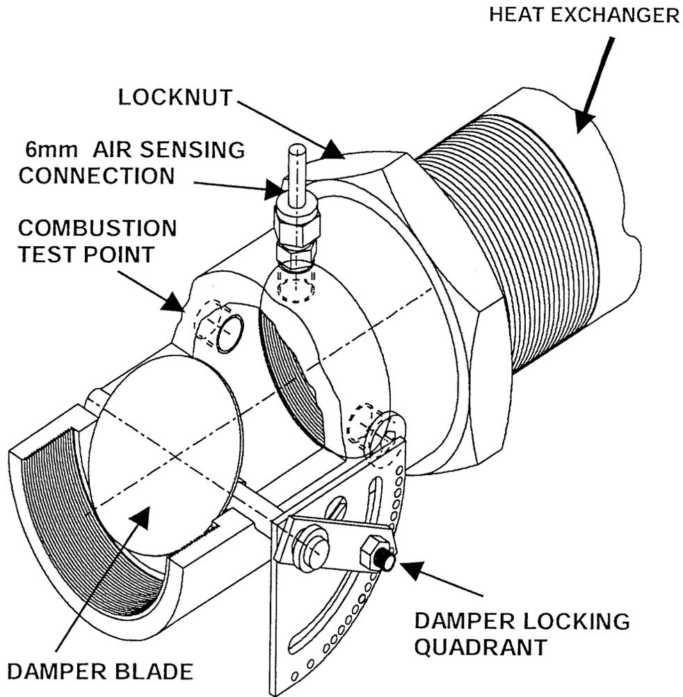
**IMPORTANT:** The damper assembly should be installed as shown with the 6 mm air sensing connection pointing upwards ( to prevent condensation blocking it ) and with sufficient clearance all around to allow Service Engineers access to set the damper quadrant and to use the combustion test point.
