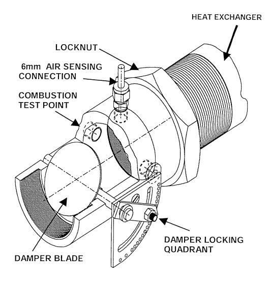
**IMPORTANT:** The damper assembly should be installed as shown with the 6 mm air sensing connection pointing upwards ( to prevent condensation blocking it ) and with sufficient clearance all around to allow Service Engineers access to set the damper quadrant and to use the combustion test point.
